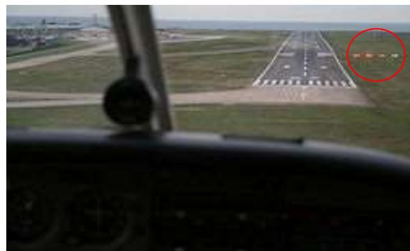
Figure 4: The Precision Approach Path Indicator
