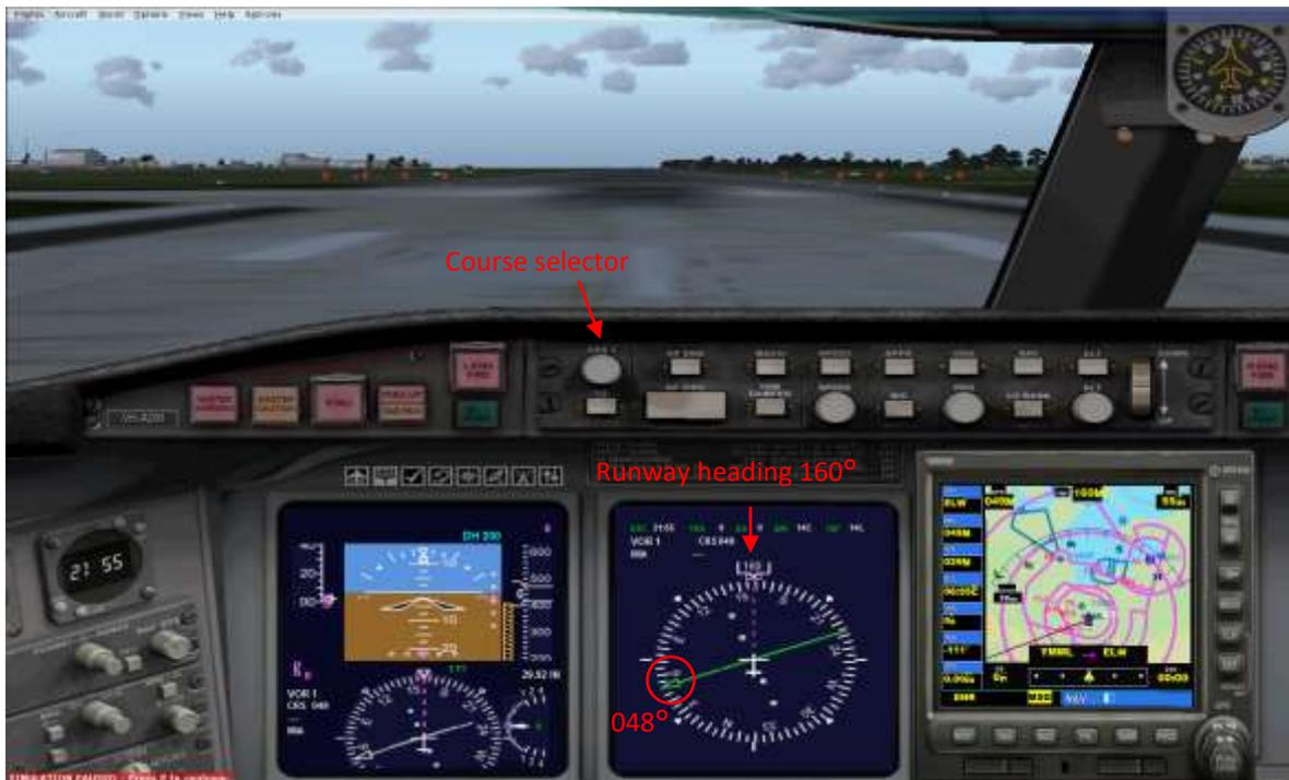
Figure 2: Navigation settings prior to takeoff
