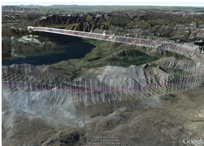
Figure 5: GE engineers designed this “highway in the sky” approach into Queenstown, New Zealand.
